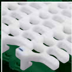
S.201Hook Open radius belt with a very low collapse factor. Can run in S- and J-curves for spiral coolers/freezers as well as normal radius applications.
