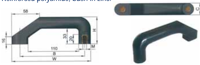
Reinforced polyamide, bush in zinc.
